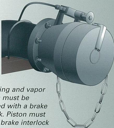
All loading and vapor headers must be equipped with a brake interlock. Piston must engage brake interlock when connected for loading.
