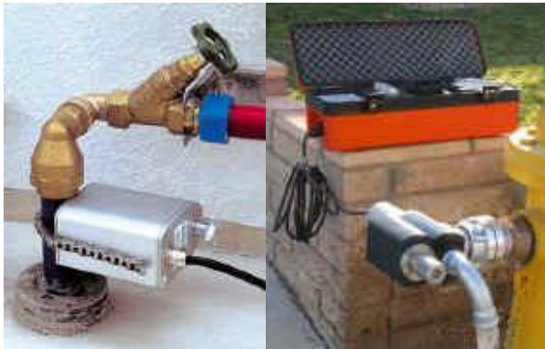
Figure: Acoustic Pipe locator. Knocker on left. Pressure pulser on right. (Source: RJM Equipment Sales, Inc.)
